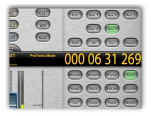
Flicking a fader quickly left or right switches the current bank up or down. This (or using the dedicated bank buttons) enables control of any number of tracks in your project.
