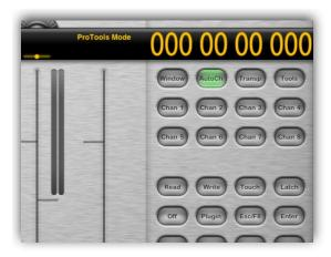
Now hold the Read, Write etc button, and tap the desired channel under AutoCh.
