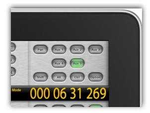
Under the time display, there's a multifunction button area. The top row of 4 buttons select which 8 buttons are shown in the the 2 rows below.
